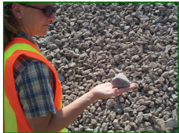
Recycled PCC Aggregate
