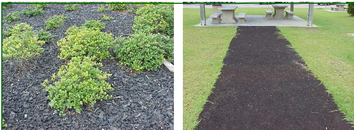
Shredded Tires Used as Loose Mulch and Sidewalk at the Colleton County I-95 Rest Area
