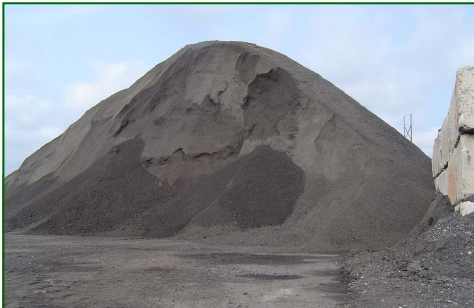
Stockpile of Recycled Asphalt Pavement (Charleston, SC)
