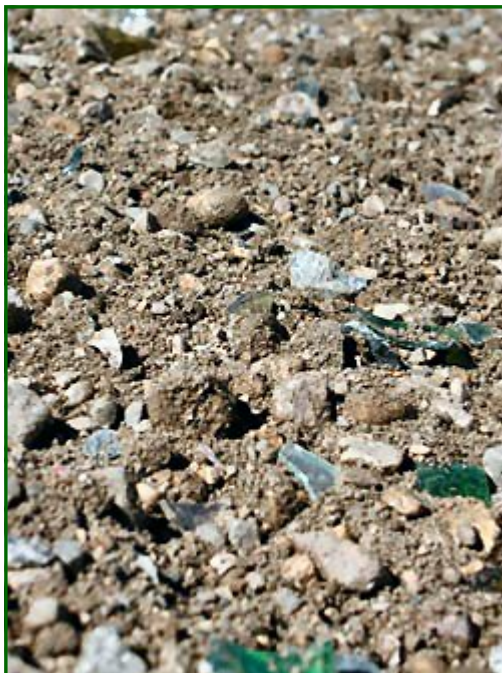
Crushed Glass as a Portion of the Aggregate for a Base Course (from www.paynesvillearea.com)
