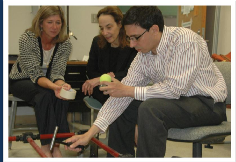
(l to r) Dr. Deb Krotish, SmartState Endowed Chair Dr. Sue Levkof, and Dr. Juan Caicedo of the SeniorSMART™ Center of Economic Excellence test a grid which was designed in the engineering laboratory to detect falling objects. The test identifies objects as they hit the grid based on vibrations detected by sensors. The grid correctly identifies the object and the location of the fallen object, then transmits the data to a computer display. This grid was originally designed to help structural degradation of bridges. SeniorSMART™ researchers are using the technology to detect vibrations following the fall of individuals in homes, retirement communities, and health care facilities.
