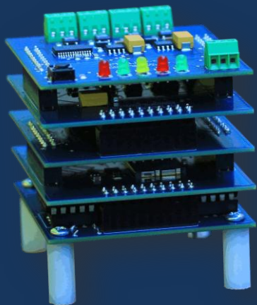
A MoteStack sensor for the Sustainable Development Center of Economic Excellence Intelligent River™ Project.
